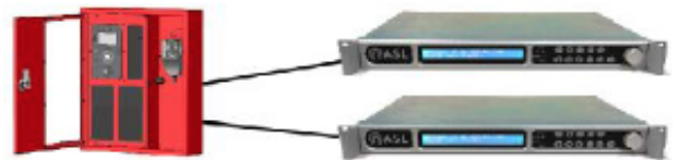
Connection to Dual Redundant Routers
