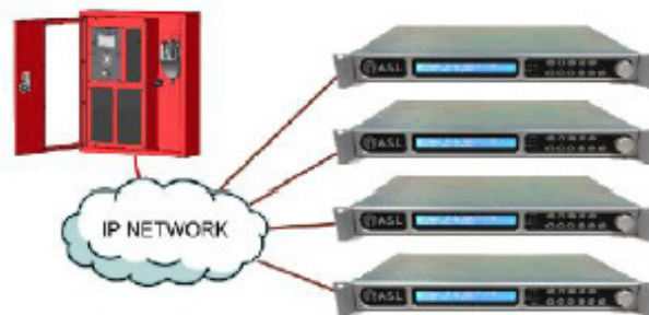
Connection to an IP Networked PA System
