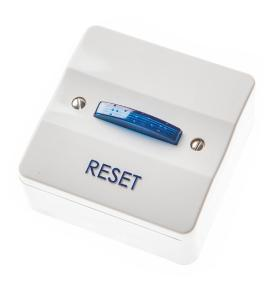
The reset unit has a blue engraved legend 'RESET'. When a call is activated the reset switch illuminates and the internal sounder activates. The call is reset by simply pressing the reset switch. The reset switch is supplied with Braille legend on the switch piece.
